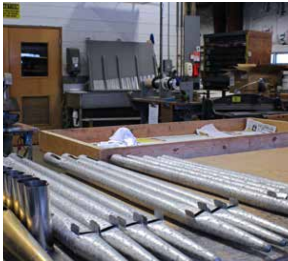
Organ pipes, formed from an amalgam of tin and lead, are one of the many components carefully crafted at the Organ Supply Industries facility.
